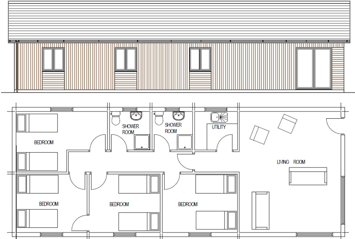
*Fig. 3: Proposed bunkhouse west elevation and floor plan*
